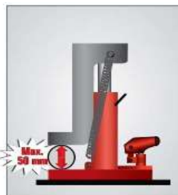
Keep the stroke max.50mm when lifting an object on the toe.
